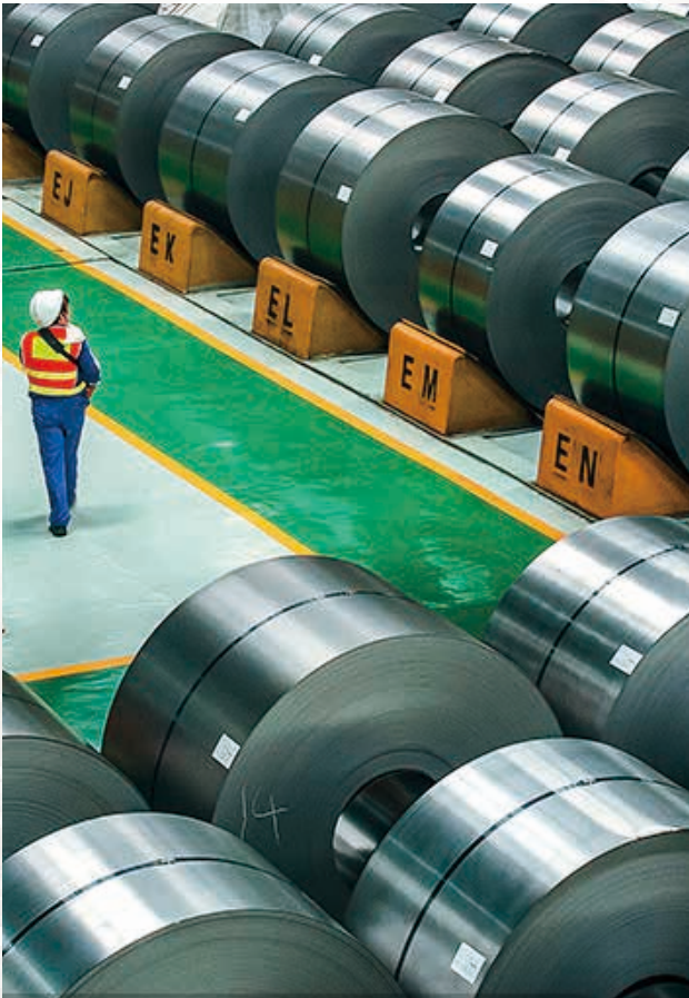
HYOSUNG (Korea) Product name: stainless steel coil Standard: ASME SA240 Material: 347H Usage: Pressure Equipment
