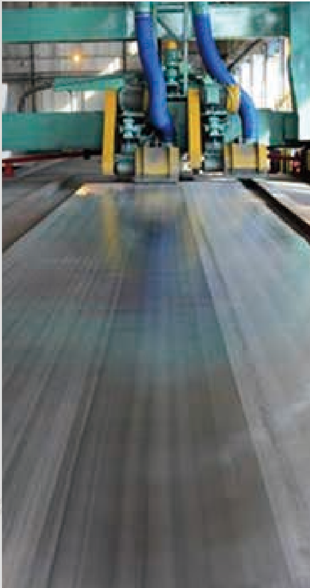
ADNOC (Middle East) Product name: Clad Plate Standard: ASME SA264 Material: SA516-Gr.70+316L Usage: Wash Tower
